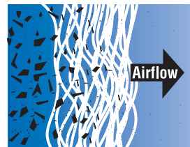
Progressive Density Media Construction
